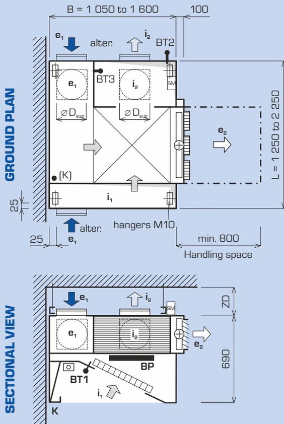
Figures show the DiNER-TN hood delivered in the right-hand design as standard. When requested, the mirror (left-hand) design can be delivered, including heating water distribution.
